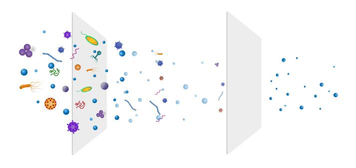
FILTER STAGE 1 Coarse dust filter G4 of 10  $\mu m$
